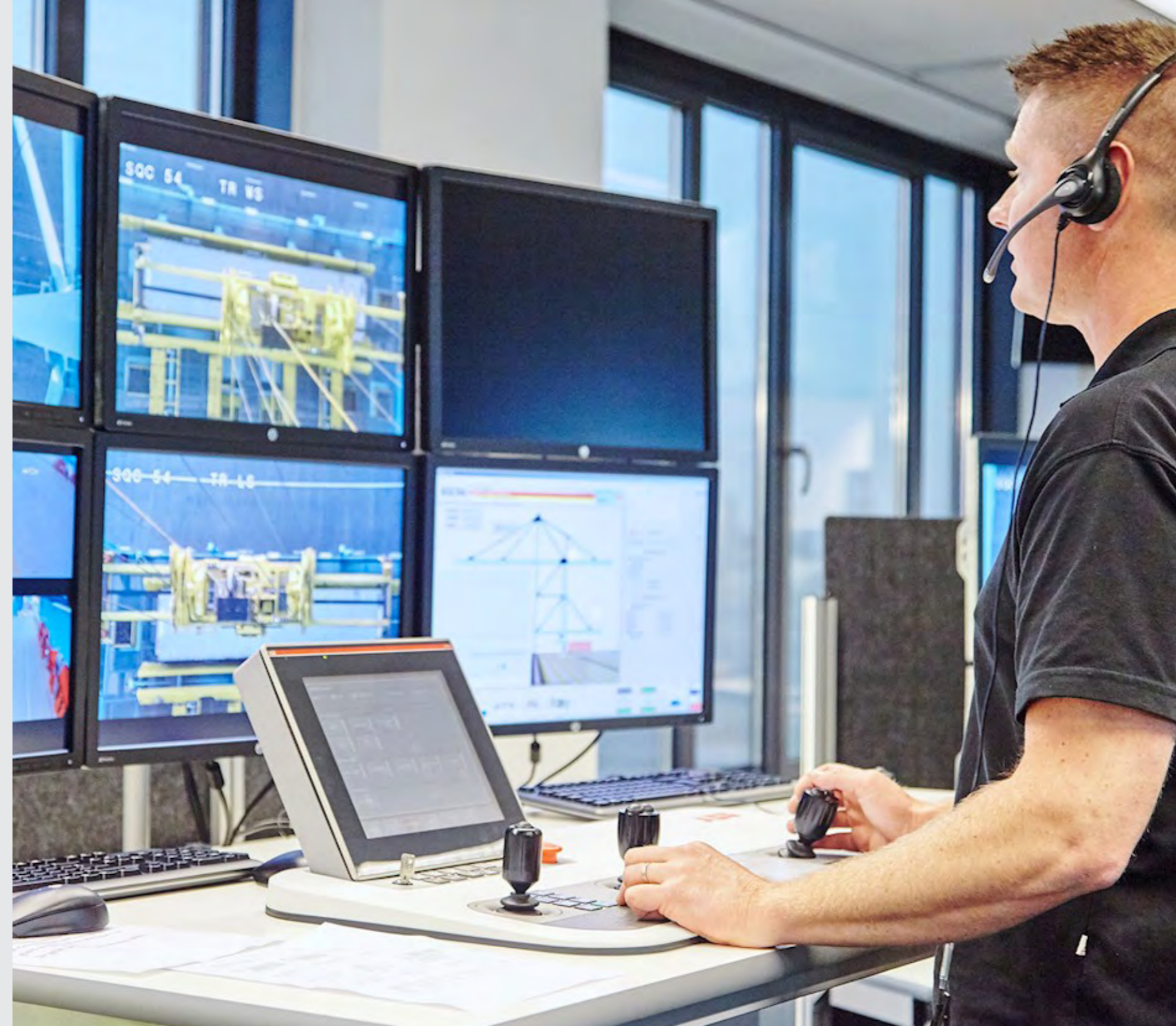
ROS working environment for gantry cranes remote operation
