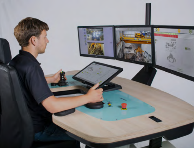
ROS working environment for gantry cranes remote operation
